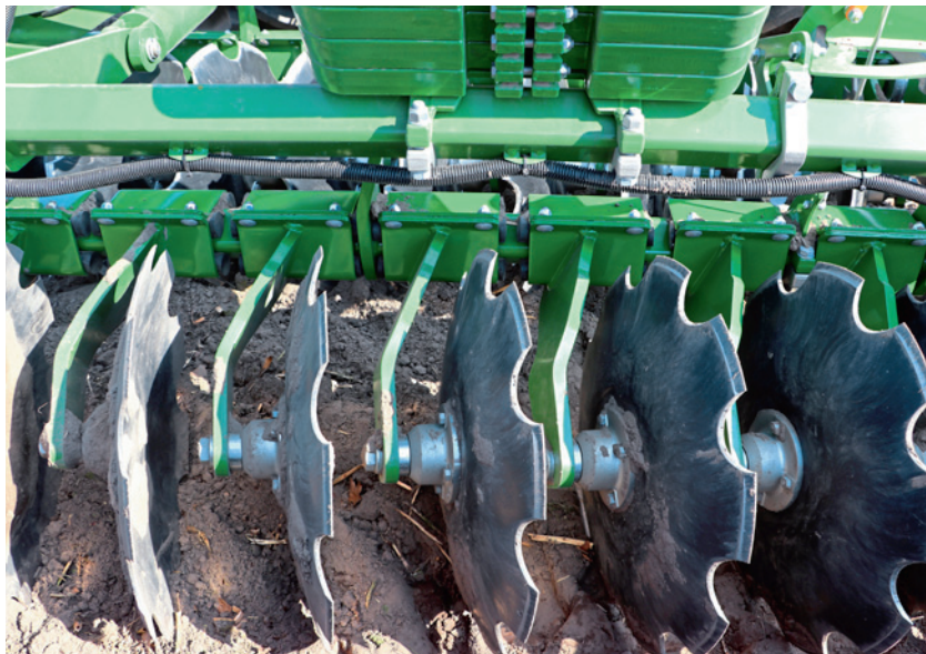
Each disc is individually attached to the frame via collar clamps. The clamps also serve as a breakback system.
