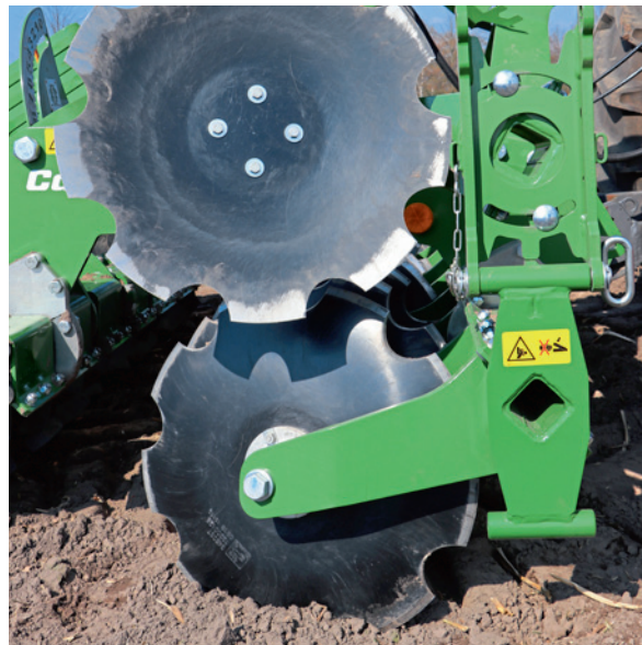
The outboard discs are folded up for transport. They also boast a precision control for depth.
