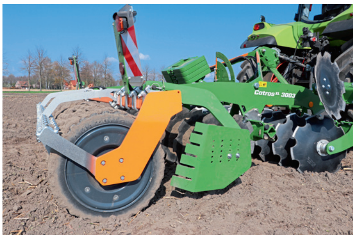
The wedge ring roller with matrix tyres gives a very good consolidation.
