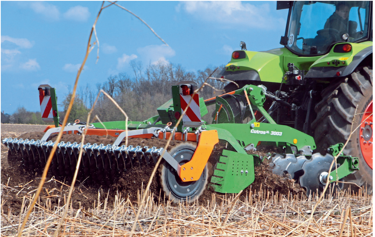
Catros XL has 610mm diameter discs designed for incorporating large masses of organic material.
