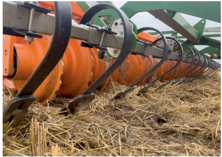
Mounted on the roller, the levelling paddles adjust automatically in depth when the roller depth changes but can be fine-tuned separately.
