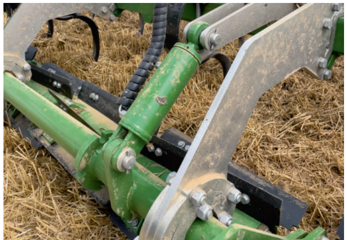
The intensity of work of the knife roller is controlled hydraulically so operators can raise it out of work conveniently.
