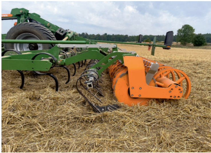
The parallelogram frame ensure consistent ground contact. Excellent.
