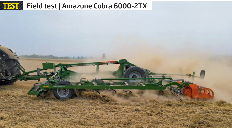
The 45 leaf-spring tines are actually arranged on 8 bars. The bars are spaced at 50-70cm, underbeam clearance is 60cm.
