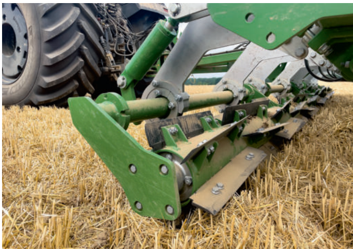
Amazone relies on a solid knife roller. The reversible knives are arranged in a V.
